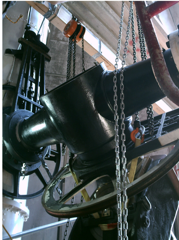
The vertical support six-roller stack assembly, patented in 1891 by Saegmuller, is reinstalled into the telescope. Photos by R.Stencel.
